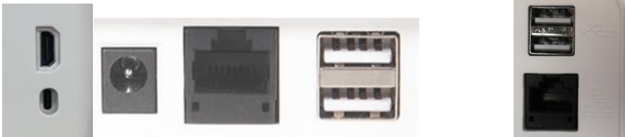
7.8./10inch device DC/NET/USB connector
