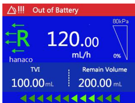
Figure 8-6 Out of battery alarm.
