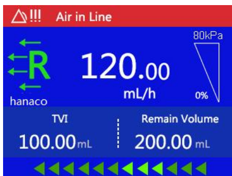
Figure 8-5 Air in line alarm.
