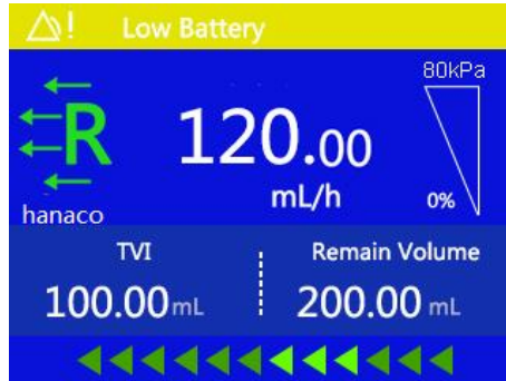
Figure 8-10: Low battery alarm.
